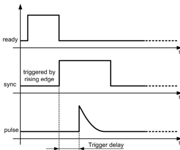
Figure 12: Signal sequence of external trigger mode, trigger on rising edge
