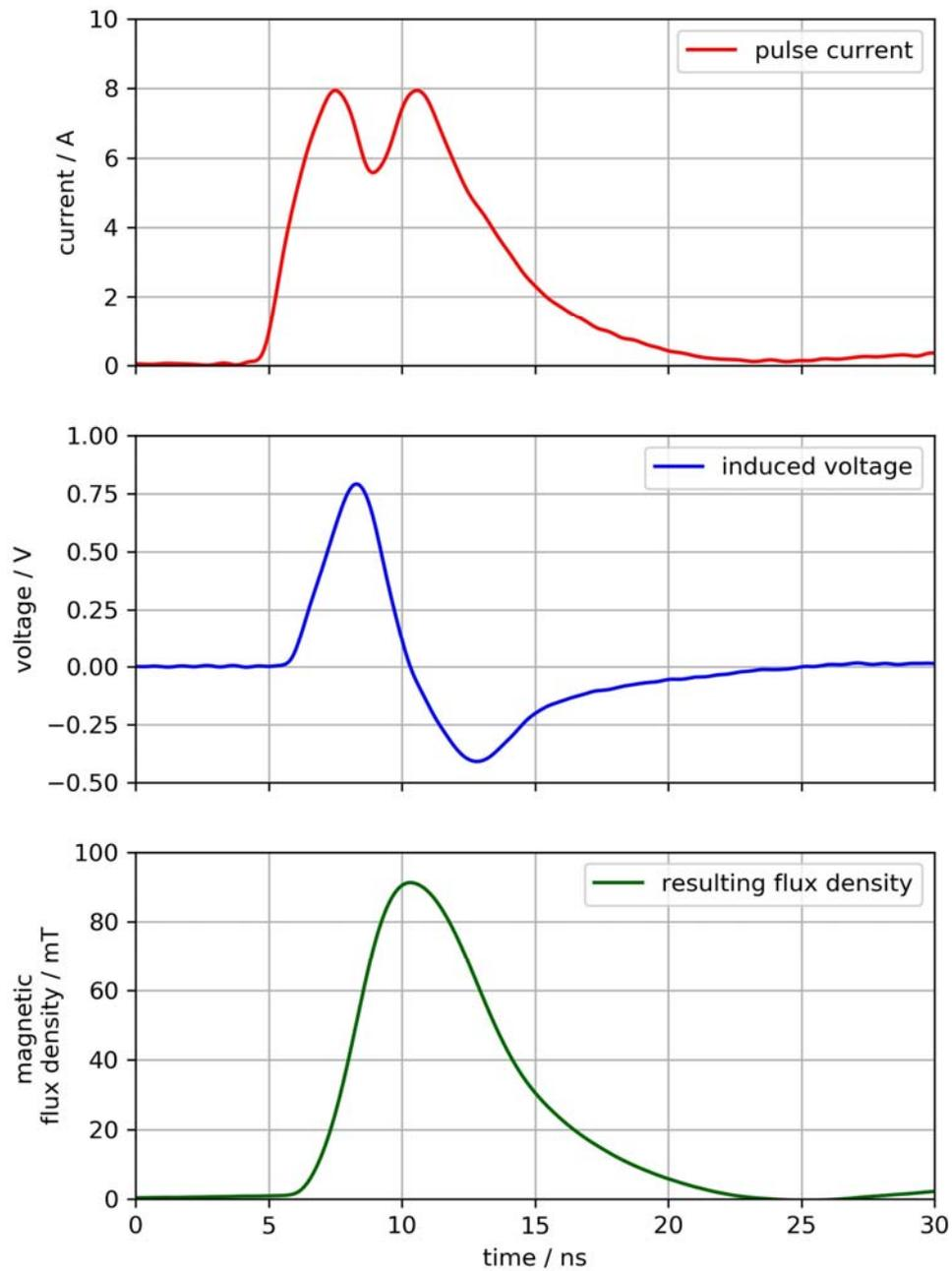
Figure 38: ICI HH500-15 typical waveform (reference setup, 500 $\mu$ m coil, 50 $\Omega$ )
