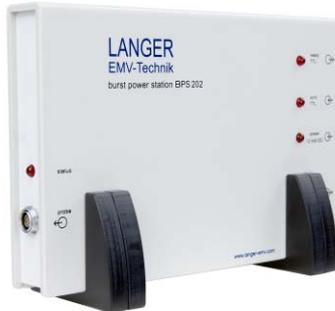
The **BPS 202** is used as power supply and control unit for the ICI probes. The control unit is connected to the user's PC via an USB interface. The provided software includes a standalone Client (**BPS 202-Client**) and a DLL for implementing automated systems. The sync TTL input allows for the synchronization of the pulse generation to external events, e. g. operation sequences of ICs.
