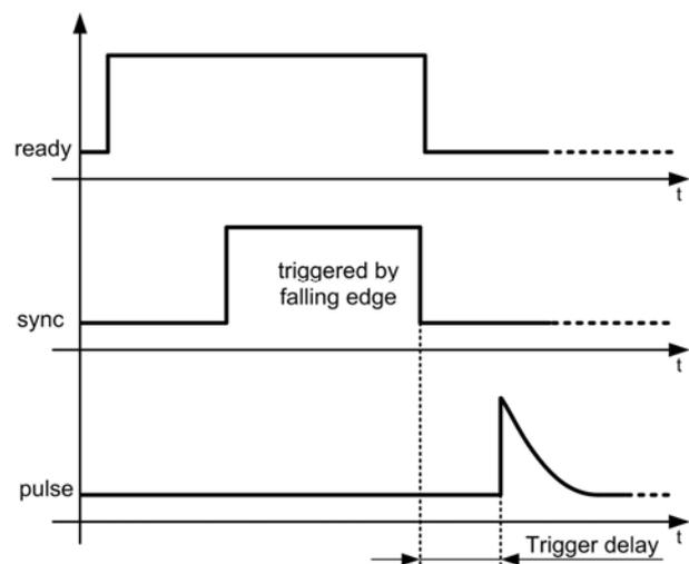
Figure 13: Signal sequence of external trigger mode, trigger on falling edge
