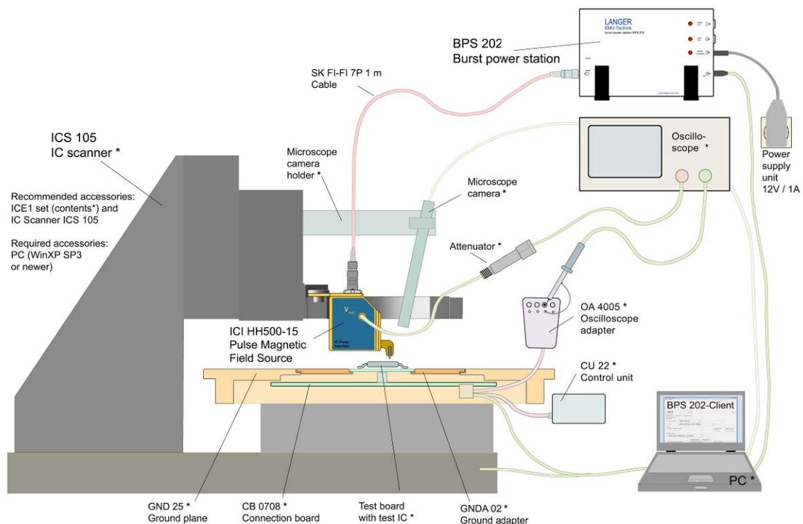
Figure 1: Setup of ICI L-EFT Set with **ICI HH500-15** probe. All devices which are not included in the scope of delivery are marked with an asterisk.
