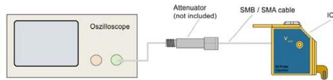
Figure 7: Setup for pulse-current measurement with an oscilloscope.
