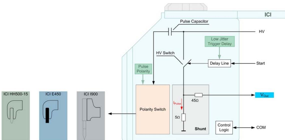
Figure 6: block diagram of the probes
