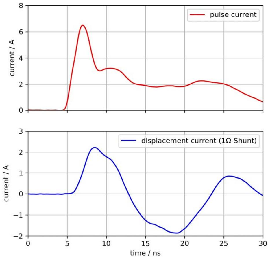
Figure 42: ICI I900 typical waveform (1Ω load, high-impedance ground connection)
