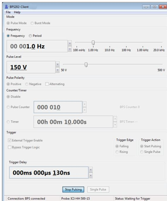
Figure 30: Trigger for **Pulse Mode**
