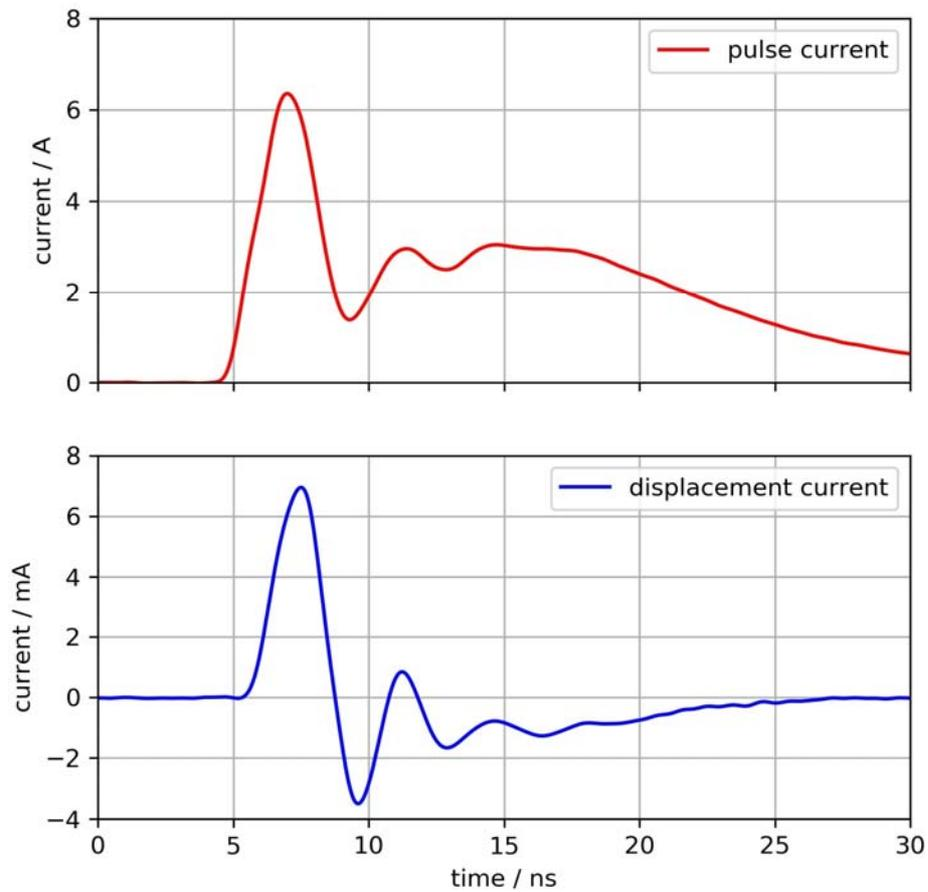
Figure 40: ICI E450 typical waveform (reference setup, 100 $\mu$ m stripline, 50 $\Omega$ )
