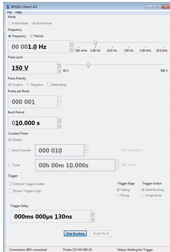
Figure 31: Trigger for **Burst Mode**
