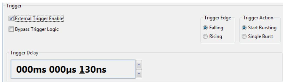
Figure 24: GUI section **Trigger** for operating mode pulse mode
