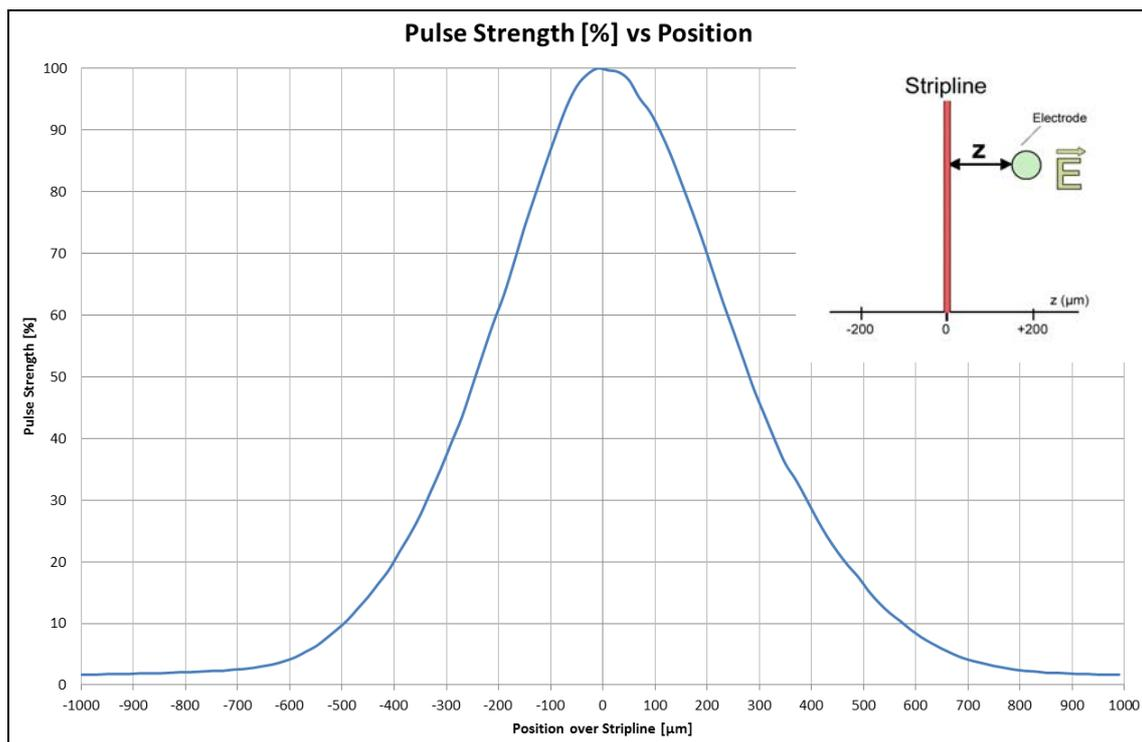
Figure 39: Relative pulse strength, scan across 100 $\mu$ m stripline
