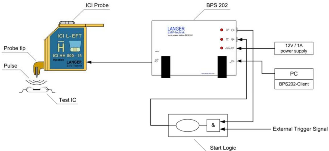
Figure 11 System setup external trigger via **BPS 202 sync TTL** input
