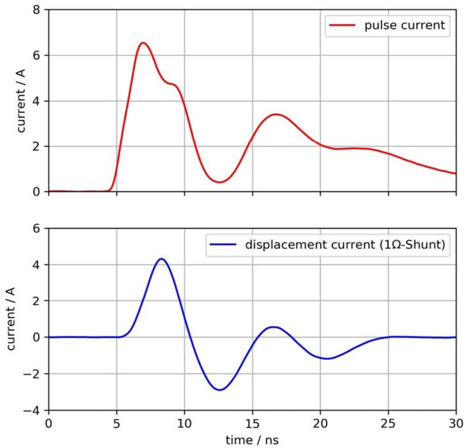
Figure 41: ICI I900 typical waveform (1Ω load, low-impedance ground connection)
