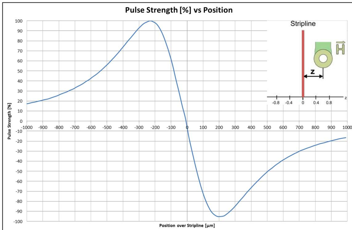
Figure 37: Relative pulse strength, scan across 100 $\mu$ m stripline
