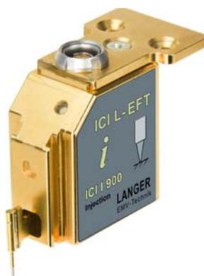
The ICI I900 L-EFT is a current pulse source with a spring loaded tip. This allows for contacting the substrate without damaging the probe tip or the test device.
