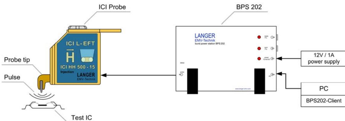
Figure 10: System setup for free running mode
